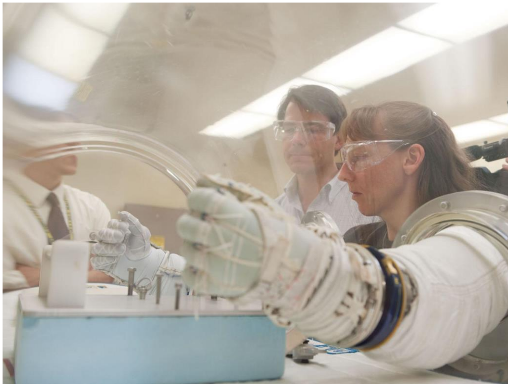
Figure 1 Astronaut Glove Challenge (2009) – Challenge winner Peter Homer observes Johnson Space Center’s Spacesuit Designer, Amy Ross, as she tests his astronaut glove prototype in a vacuum chamber. Image credit NASA
