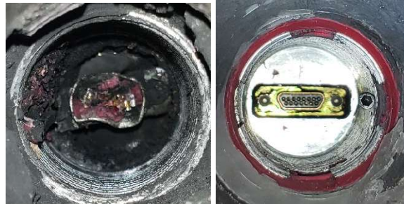
Figure 3: Side-by-Side Comparison of Recovered Projectiles with Gun Gas Leakage (L) and without Leakage (R)
