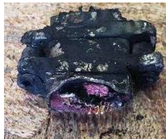
Figure 4: Connector & Shorting Plug Melted by Gun Gasses
