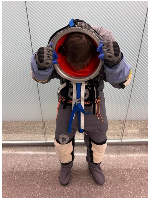
Figure 10 Neck ring over head (careful not to scrape head on ring bolts)
