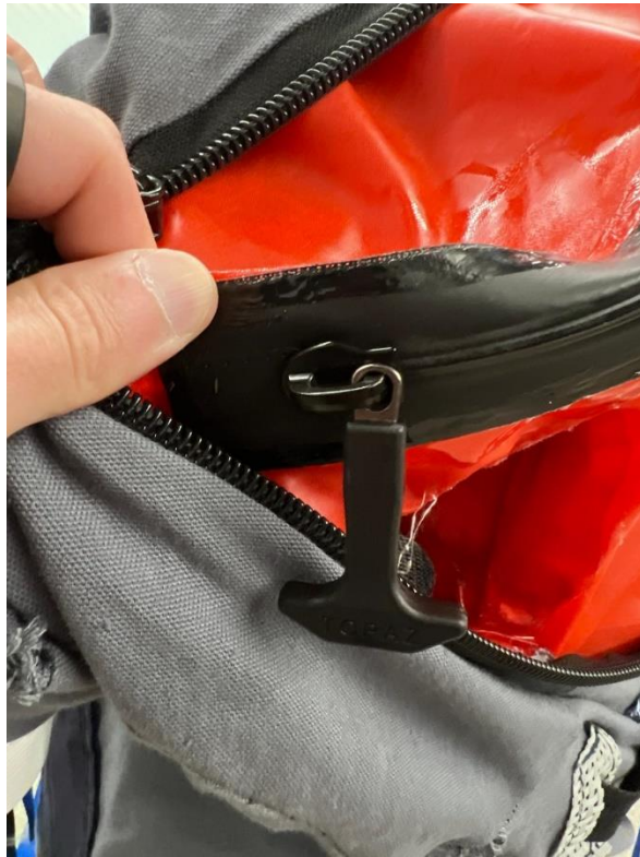
Figure 12 Visually verify bladder zipper is fully closed
