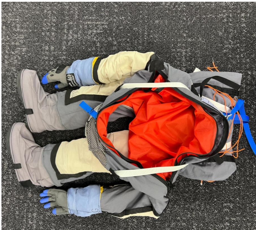
Figure 3 Undo the back buckle and unzip the two suit entry zippers
