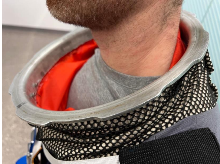
Figure 18 Helmet ring clear of any obstacles
