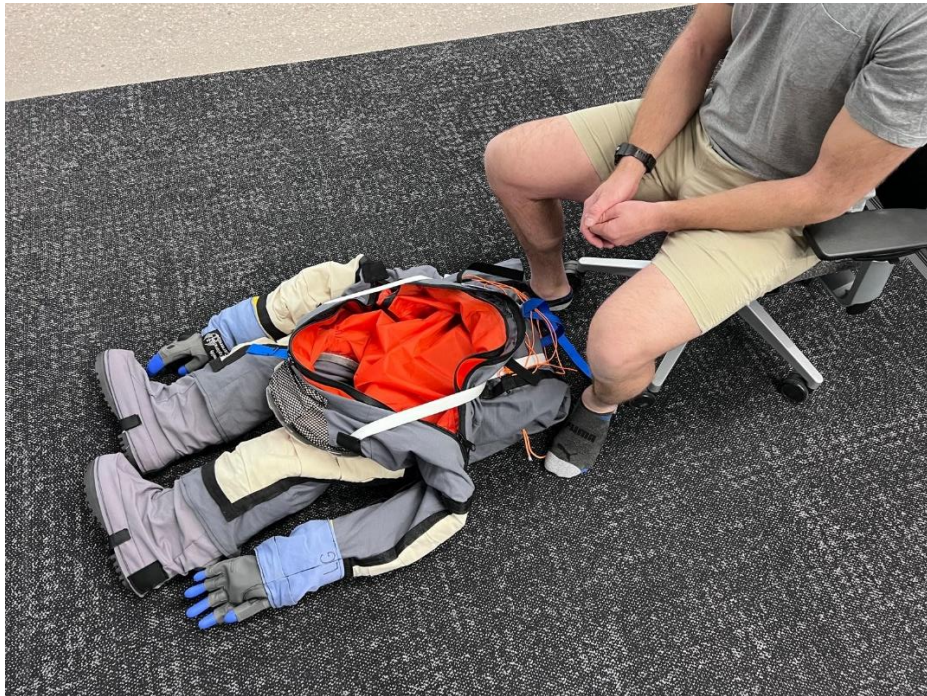
Figure 4 Participant should now be seated for suit ingress at the head of suit
