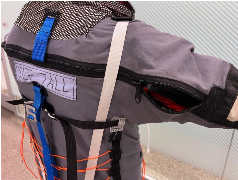
Figure 13 Zip restraint layer closed
