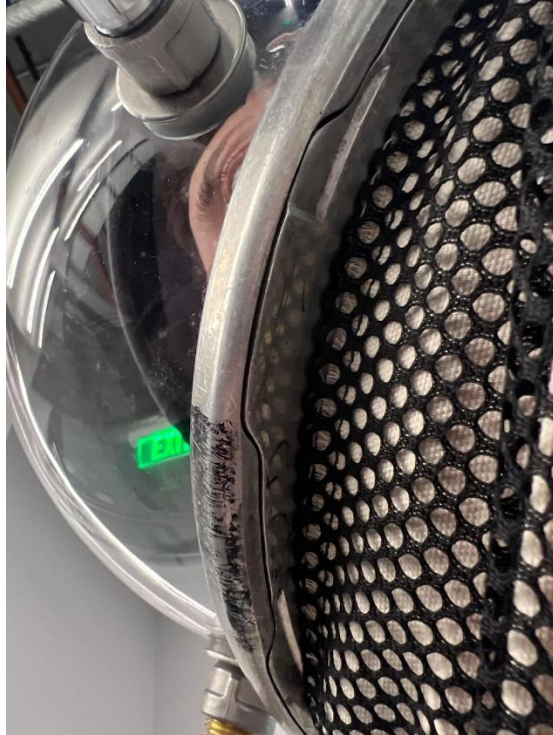
Figure 19 Place helmet over head and engage to the locked position (push down and clockwise)
