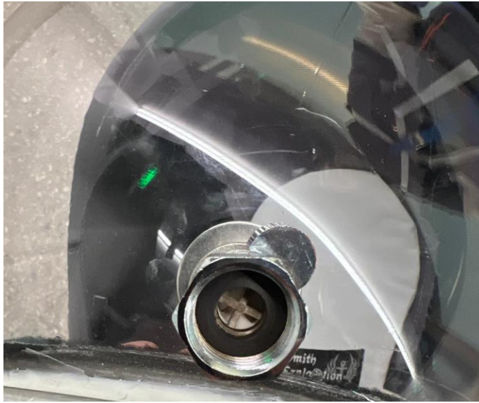
Figure 16 Helmet valve to the open position, visually confirm its open
