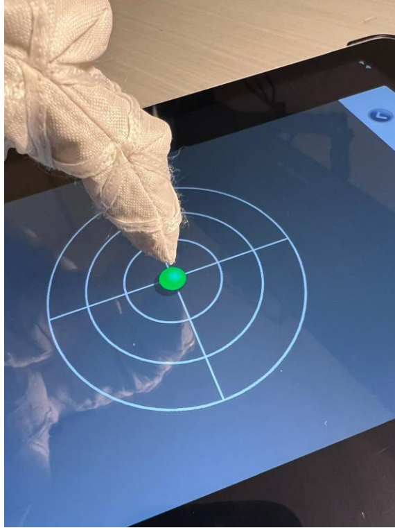
Figure 4 When gloved finger taps touchscreen with fingertip, there is no response on the screen
