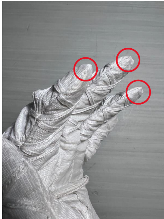
Figure 3 Fingertip fabric sewn seams circled in red
