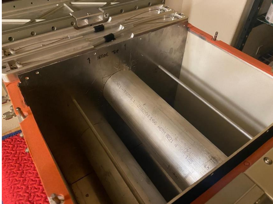
Figure 5 View inside the sorbent bed where the three sorbent tubes are found.
