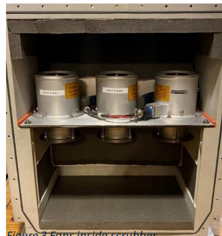
Figure 3 Fans inside scrubber
