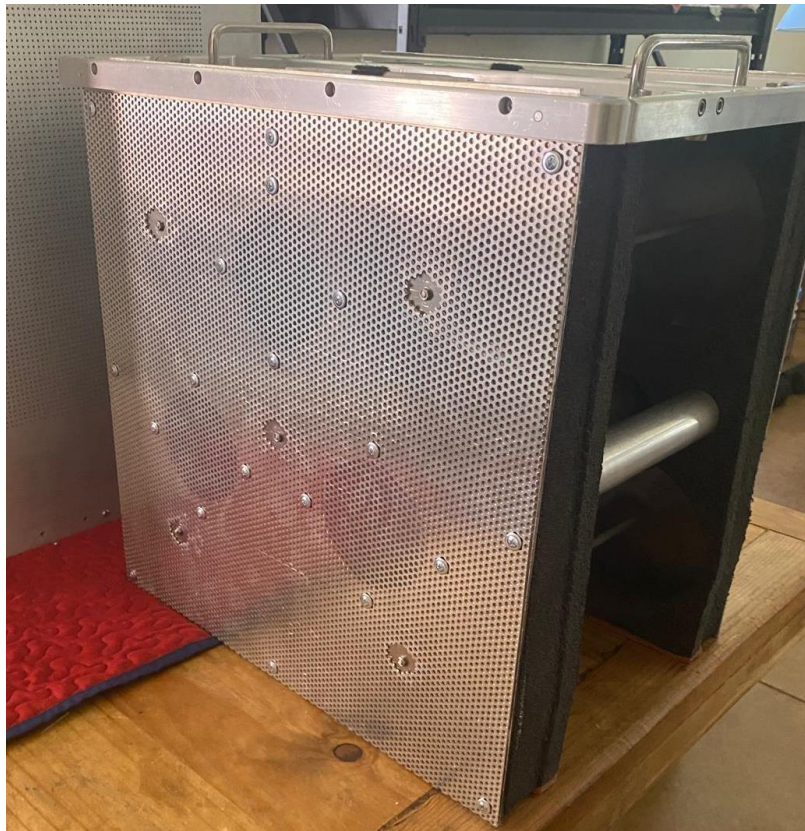
Figure 14 View of sorbent bed outside of scrubber
