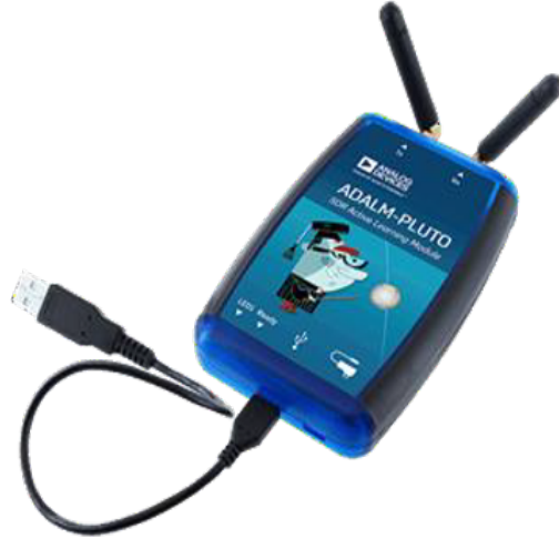
Figure 5: Analog Devices ADALM-PLUTO SDR used in OTA experiments.
